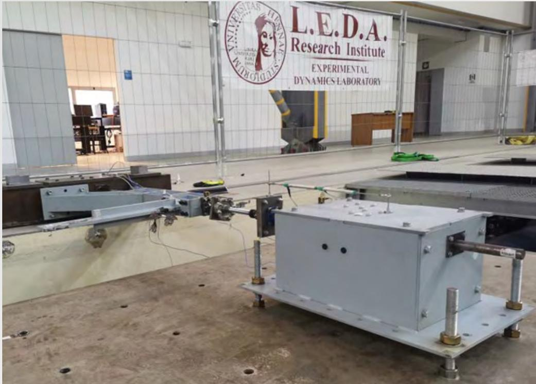
Mechanical inerter device
