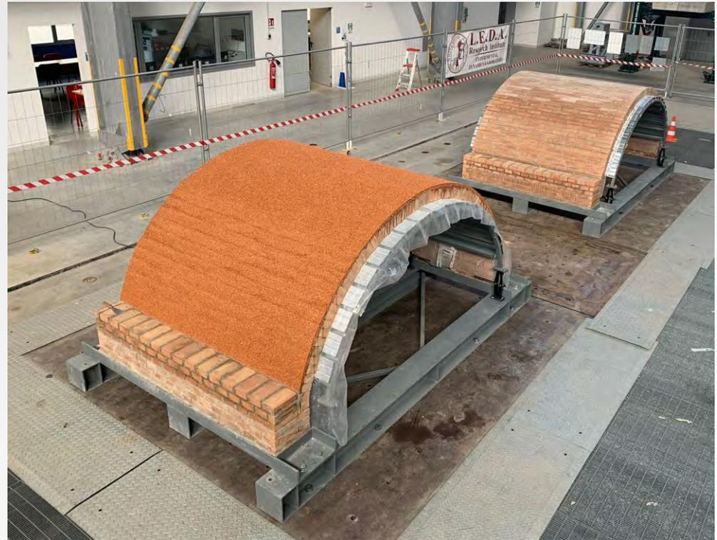
Barrel vaults strengthening with hemp fibres
